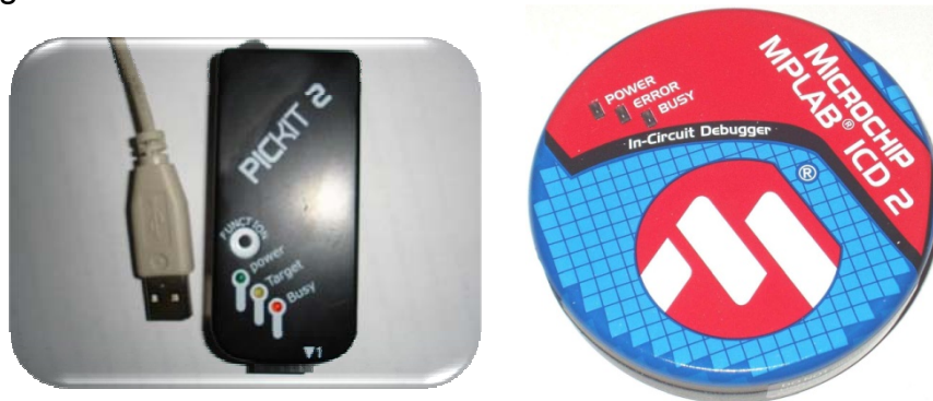
Figuur 9: MPLAB pickit2 & ICD2 programmer
